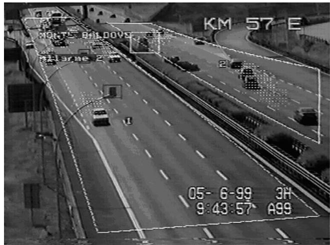
Figure 1. Real-time video detection of a stopped vehicle
