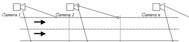
Figure 3. A schematic representation of the discrete rhythm of camera views located on a road section.
