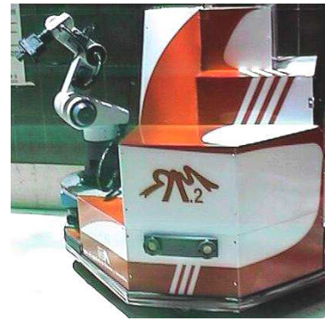
Figure 3. The mobile robot RAM-2. It is equipped with a robotic arm, and several sensors as a laser scanner, ultrasonic sensors, and a CCD camera.
